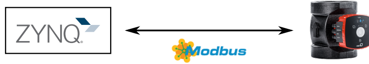
Figure 5.13: System emulation with Modbus-based communication between Xilinx Zynq computational unit and KSB Calio pump (sources: Xilinx, www.modbus.org , www.ksb.com ).
