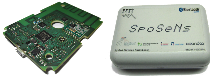
Figure 3.4: Hardware and enclosure of the final wearable sensor device SpoSeNs Node .
