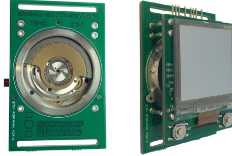
Figure B.3: Bottom view on the harvester and top view on the display of the assembled EternAlyzer .
